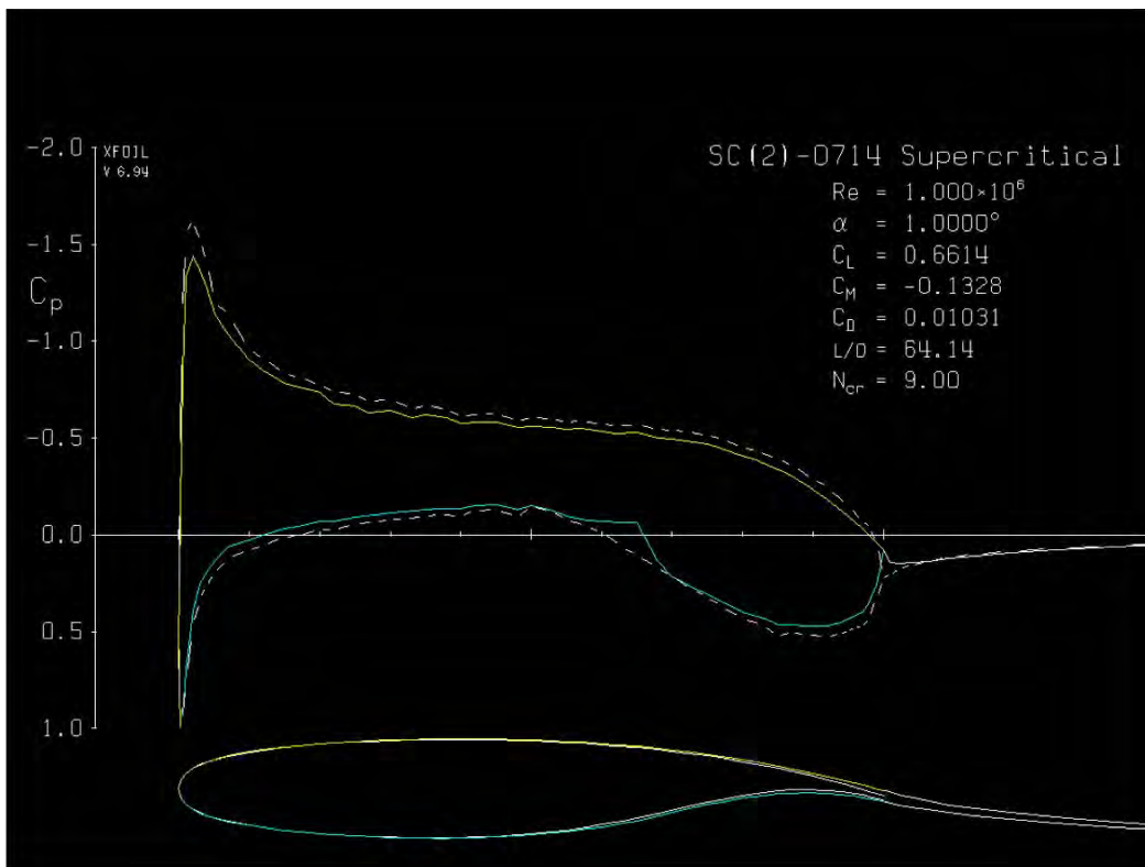
Figure 12: The NASA SC(2)-0714 Airfoil in XFOIL
